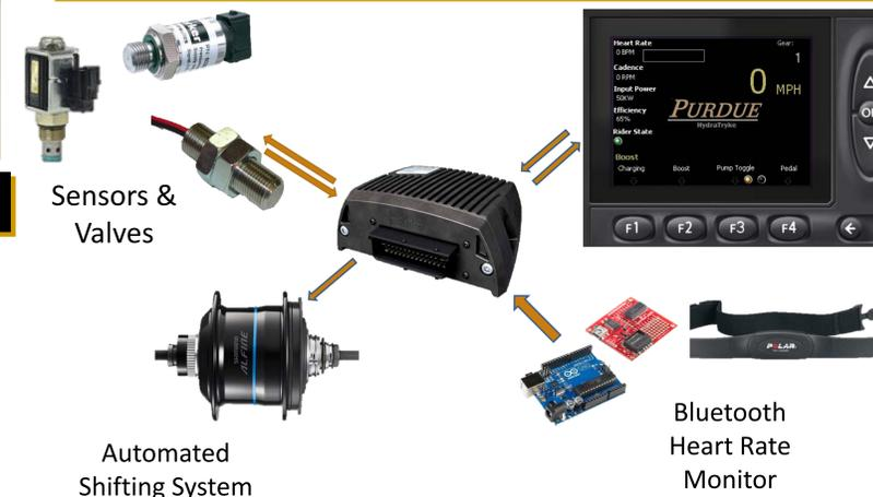
The heart rate monitor allows the user to customize their workout to fit their specific need. The sensor tells the IQAN the state of the rider so that the rider knows if their heart rate is in the target range or not. Depending on whether or not the rider's heart rate is in the target range, the IQAN can automatically shift to better meet the fitness level.
