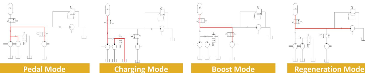
The first function is pedaling, which enables the rider to manually power the bike. The next function requires the rider to charge the accumulator before each race. After charging the accumulator the boost function may be used to propel the vehicle forward. Lastly, a regeneration function will allow the rider to brake the vehicle and store some of the energy by recharging the accumulator.
